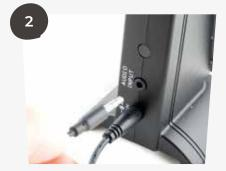
Connect to an audio source using the cables provided.
